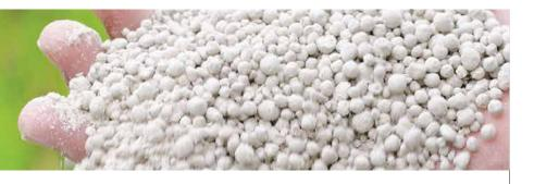
"Perlite is a type of volcanic amorphous rock with masses of water droplets formed by cooling of lava formed in acid phase in the magma. Perlite is an insulating material. Perlite is a radioactive-free mineral. Perlite is an inorganic substance. It does not lose its property at high temperature and prevents the spread of fire with such property. Perlite contains plenty of air voids."
